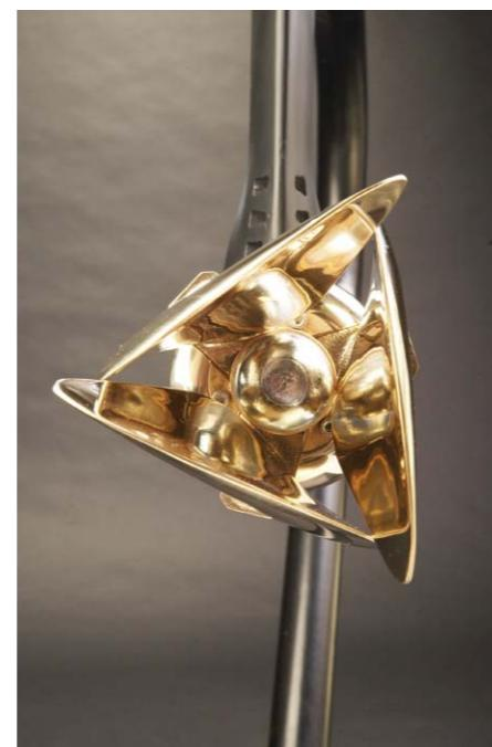
Brunton's Varifold 3 blade (made by SPW in Germany) is a popular choice as it gives a combination of minimum drag with power. Photo Bruntons
