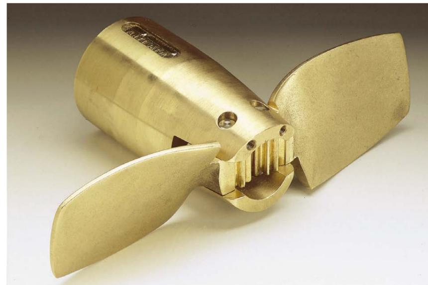
The Volvo sail drive folding model is designed for ultra low drag; important when there's two of them. *Photo Volvo Australia*
