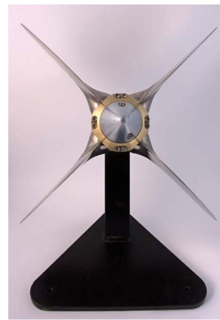
Darglow UK build a range of Featherstream propellers that use a cassette to vary their pitch. Suitable for mono or multi-hulls up to 55ft the come in 12-20 inch diameters with 3 or 4-bladed models for both shaft and saildrive. The company offers discounts for cat owners buying two props. Photo Darglow UK
