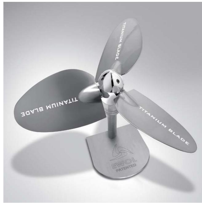
Ewol's prize winning titanium feathering model can be micro adjusted to maximise engine revs while offering a high performance under sail. Photo Ewol Italy
