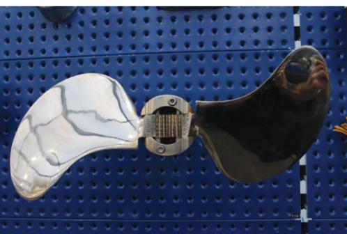
Volvo range of folding propellers comprise 2, 3 and 4-blade models for both shaft and saildrives; and of course are built specifically for their engine gear ratios for maximise performance. *Photo Kevin Green*
