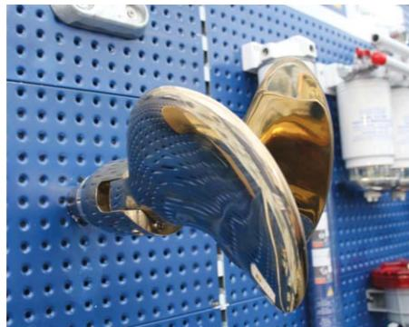
Volvo range of folding propellers comprise 2, 3 and 4-blade models for both shaft and saildrives; and of course are built specifically for their engine gear ratios for maximise performance. *Photo Kevin Green*
