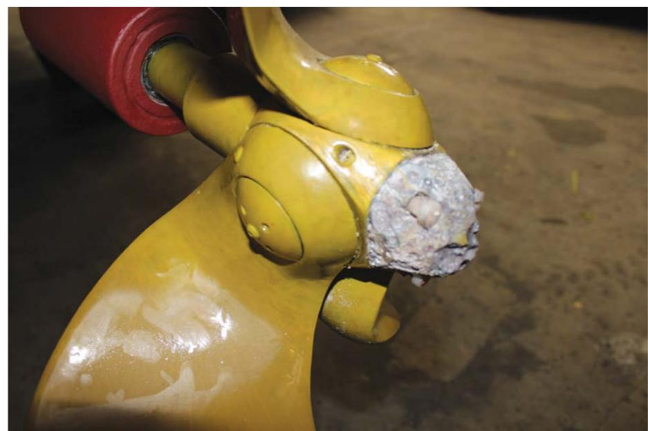
Regular maintenance and replacement of anodes is important to combat electrolysis.
