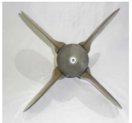
**left:** Sydney made Hydralign claim the largest range of feathering propellers in Australia – offering 2, 3 and 4-blades, ranging up to 36 inch diameter, including specialist ‘aperture’ models for classic yachts. *Photo Hydralign*
