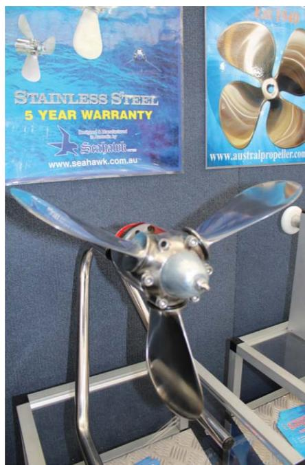
above and right: Brunton's in conjunction with SPW Germany supply the Varifold range that comes in 2, 3 and 4-bladed folding models, offer ultra-low drag. Photo Bruntons
