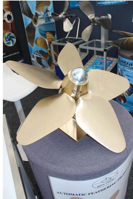
American PYI's Max-Prop five bladed Whisper generates a lot of thrust while automatically feathering to minimise drag.
