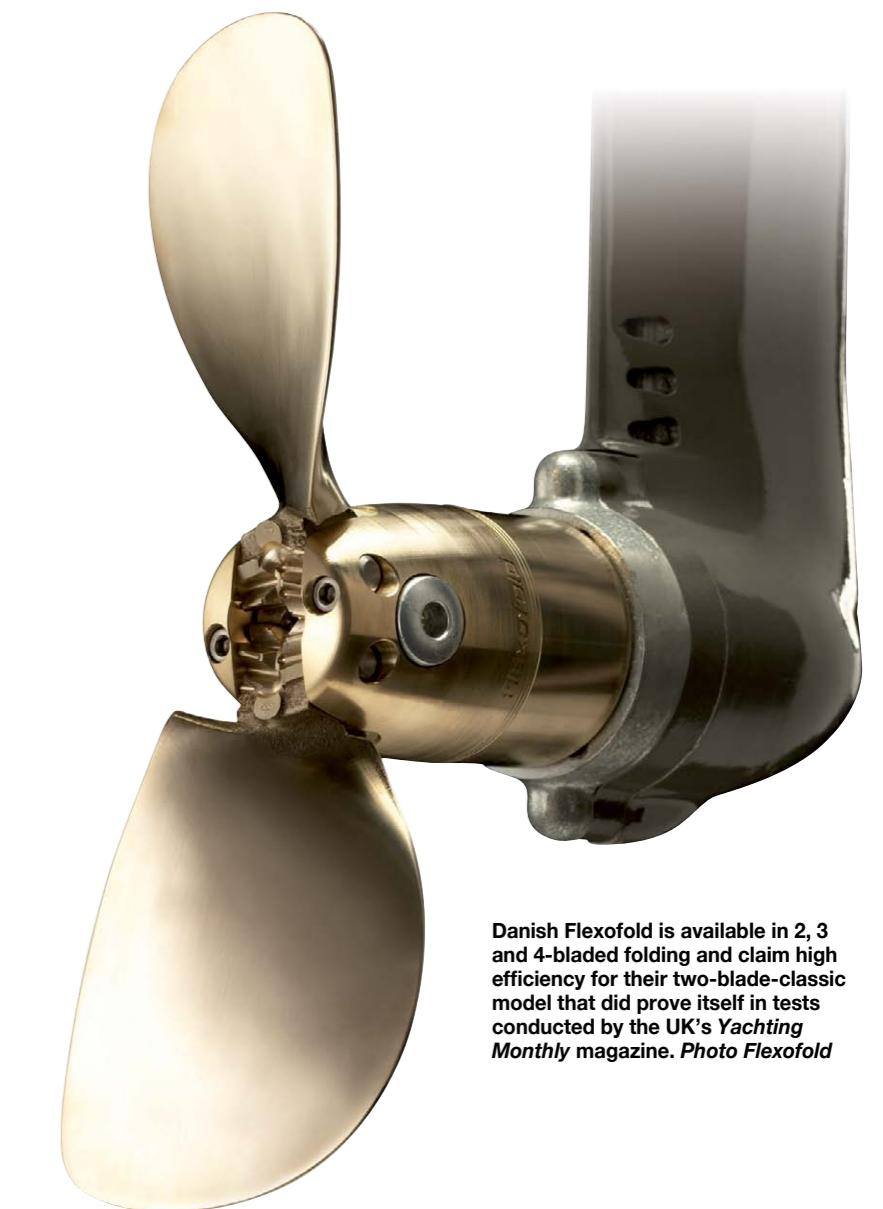
Danish Flexifold is available in 2, 3 and 4-bladed folding and claim high efficiency for their two-blade-classic model that did prove itself in tests conducted by the UK's *Yachting Monthly* magazine. Photo Flexifold
