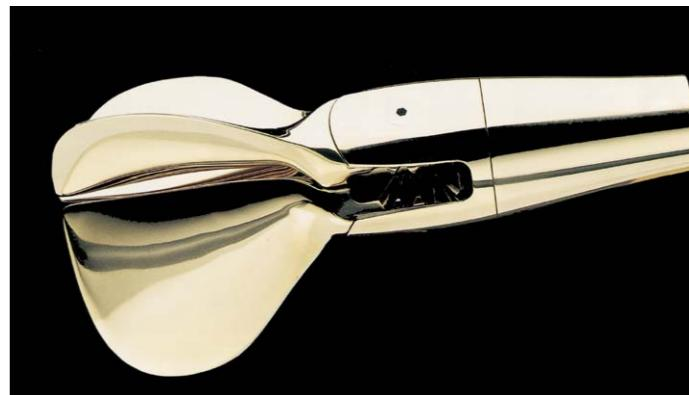
models via an outer Micrometric Pitch Setting Device allowing the precise inclination of blade with angled steps of 0.25°, corresponding to variations of about 30-50rpm at max throttle. It was interesting to read Nigel Calder's article in Australian Yachting which showed that fitting a fuel meter – as most
